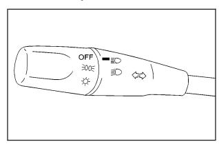
The lever on the left side of the steering column operates the exterior lamps.
